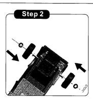
2.Insert the rear wheel axle through washer, wheel, plastic ring into the body, tighten using a cotter pin.
