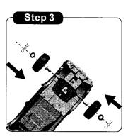
3. Assemble the two front wheels, insert the plastic ring, wheel and washer, tighten using a cotter pin.
