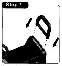
7.Insert the backrest over the hole in the rear of the body,be certain the backrest is completely seated.
