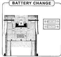
Trun over the car body, and find the battery house. Loosen the screws with a screwdriver. Put 2 AA batteries in the battery house, then tight the screw with a screwdriver.
