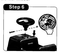
6.Loosen the bolt and nut in the steering wheel first, then place the steering wheel over the J-shaped stick, insert the bolt and tighten the nut with a screwdriver.
