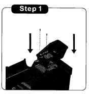
1.Place the anti-tumble shelf into the rear of the body,tighten with 2 scews by a screwdriver (not included).
