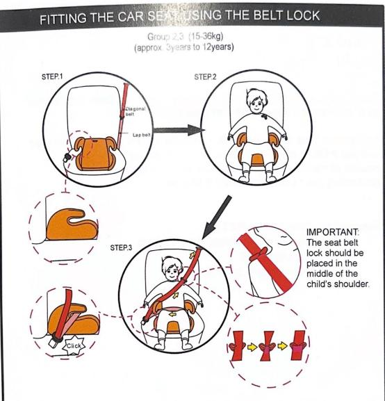
Step1. Place the booster seat on the vehicle's seat ensuring it is firmly pressed against the car seat backrest.
