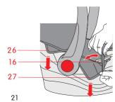
Step8: Take out lap sections of the adult safety belt from both lap belt guides(fig. 16) as shown
