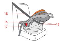
• Place the diagonal belt(fig. 18) in the diagonal seat belt guide(fig. 19) at the back of the seat.
