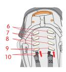
There are four sets of slots on the shell(fig. 6,7,8,9.), open the belt buckle, pass the strap(fig.10) through the slots to fit the child's height.
