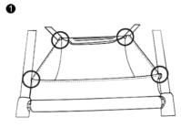
Fit the baskets fixing straps with hooks on frames (4 positions) and fit the fixing strap onto footrest (3 positions), and wrap the back fabric cover with rear crossing tube by velcro ( diagram 1).
