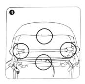
2.Fit on the front sleeve of seat cover onto the leg-rest tube and close by velcro, then close the velcros on front and back crossing tubes, tighten the support webbing by metal buckle in the middle ( diagram 4).
