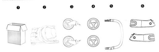
Open the package carton and take out the frame with fabric covers, front wheel, rear wheel and front bumper bar, and car seat adapters.
