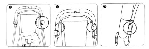
1.Slide the seat fabric cover side wings fixing rod onto the slot of handle tube ( diagram 1), fix the top support rod onto connector and hang on by elastic strap ( diagram 2 and diagram 3) .
