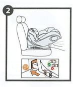
2. Push the car seat as far as possible into the seat and check its correct installation the correct installation indicators should turn green.
