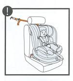
IMPORTANT: The Top Tether strap must not pass over the vehicle's headrest. It should pass under the headrest - if this is not possible, remove the headrest (check whether this is allowed according to the vehicle's manual).
