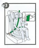
3. Place the child in the car seat. Guide the shoulder belt through the green shoulder belt guide. Guide the car seat belt through both waist belt guides. Fasten the car seat belt. You will hear a characteristic "click".
