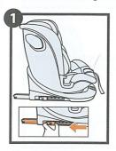
1. Install the car seat forward-facing using the ISOFIX connectors. If the car seat is already installed using the ISOFIX connectors, change its position to forward-facing using the easy spin mechanism.
