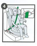
4. Place the child in the car seat. Guide the shoulder belt through the green shoulder belt guide. Guide the car seat belt through both waist belt guides. Fasten the car seat belt. You will hear a characteristic "click".
