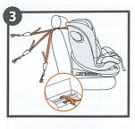
Attach the mounting hook of the strap to the vehicle's attachment point (it is necessary to refer to the vehicle's manual).
