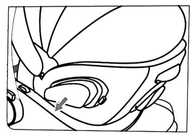
The "Linear Side-impact Protection" (L.S.P.) is built into the car seat. This system enhances the safety of your child in the event of a side crash. In order to achieve the best possible protective effect, unfold the L.S.P. (24) as far as possible towards the vehicle door closest to the car seat. To Release the L.S.P push the marked area(25) on the L.S.P. If it's not possible to completely unfold the L.S.P. with a closed vehicle door, you may as well use the infant car seat with a closed L.S.P.
