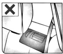
WARNING! Never use the car seat on a vehicle seat with an activated front airbag. This does not apply to so-called side airbags.
