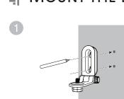
· Check for reception strength and camera angle before drilling the holes.
