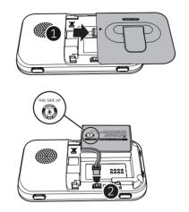
• Make sure the label THIS SIDE UP is facing up while inserting the battery
