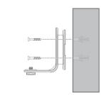
Align the wall mount bracket and screws with the holes in the wall as shown. Tighten the screw in the middle hole first, so that the wall mount bracket position is fixed. You can tighten the other screw in the top hole.
