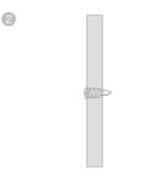
Drill two holes in the wall. If you drill the holes into a stud, go to step 3.
