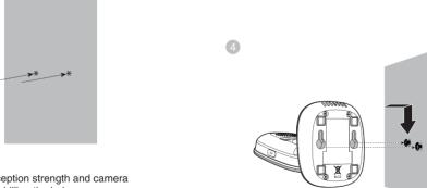
Align the wall mount holes on the baby unit with the screws on the wall. Slide the baby unit down until it locks into place.
