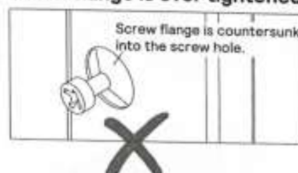
Screw flange is over tightened
