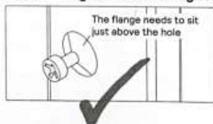
Screw flange is not over tightened
