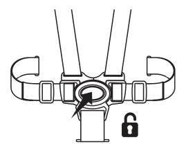
**5.** To adjust the shoulder and waist straps length, move the sliders as shown.
