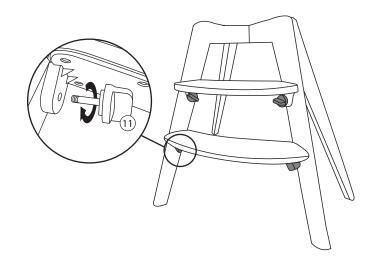
**6a.** Position the seat unit (1) over the assembled wooden legs. Align the holes ensuring that the seat and the footrest are on the same side.
