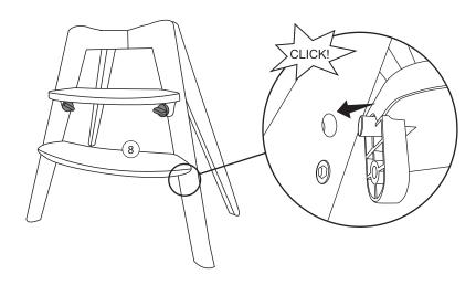
**5b.** Insert the a bolt (11) into the hole allocated on the inside of the footrest. Turn the bolt clockwise to tighten and secure. Repeat for the other side.
