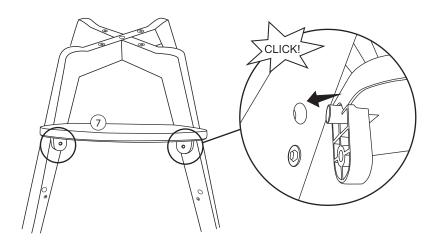
**4b.** Insert the a bolt (11) into the hole allocated on the inside of the footrest. Turn the bolt clockwise to tighten and secure. Repeat for the other side.
