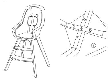
**6b.** Insert screws (9) into the holes from the underside of the wooden legs and tighten with allen key (12). Be careful not to over-tighten.
