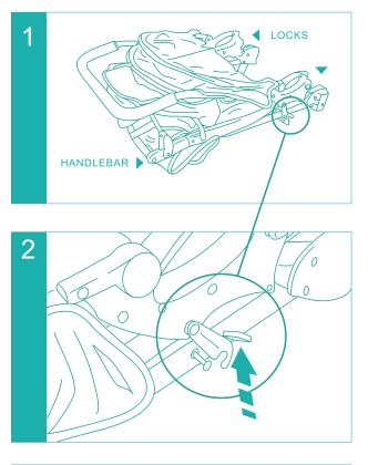
Lay the chassis down flat with the two locks facing up. Remove all packaging materials from the chassis.
