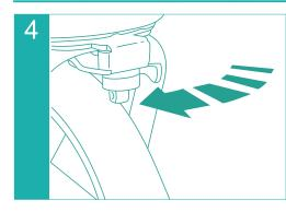
The front wheel can be unlocked to allow it to rotate, giving greate mobility. It is recommended that this is only done on smooth surfaces, and that the wheel is locked when on uneven surfaces to prevent vibration.
