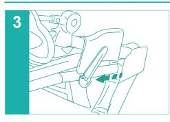
Attach the folding latch before carrying the three-wheeler.
