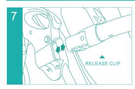
Insert the ends of the bumper bar into the slots on the frame, with the release clips underneat Check the bar is securely in plac buy pulling it. To remove the bar push in the release clips on both sides and pull the bar out.
