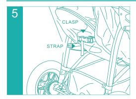
The seat back can be lowered by loosening the strap until the desired seat height has been reache or by pressing the buttons on the clasp. To raise the seat, hold the fastened clasp and pull the strap.
