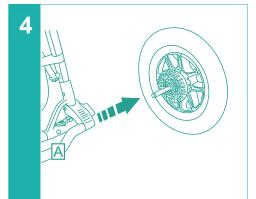
The front and rear wheels have been designed to be easily removable for more compact storage of the three-wheeler. To remove the rear wheels lift tabs (A) on the pushchair chassis, as you pull the wheels at the same time.
