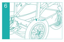
The tyre pump is secured in the shopping basket. The threewheel's tyres are semi-inflated. You should pump them until they are inflated to 28psi. Do not ove inflate them.
