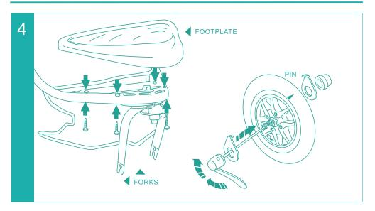
Remove the plastic packing from the front forks and dispose of safely. Remove the outer nuts and washers from the wheel's axle. Fix the front wheel into the slots on the front forks. Slide the washers onto the axle, fitting the pins into the holes on the forks.
