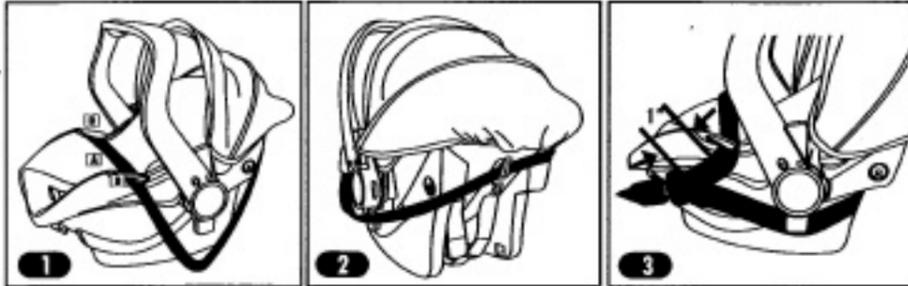
2. Put lap belt (A) over car seat and under the two belt hooks (B). (Fig .1)
