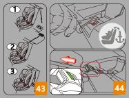
Finally check the child seat is fixed stable on the vehicle seat. If you experience any shaking movement you must tighten the belt again.
